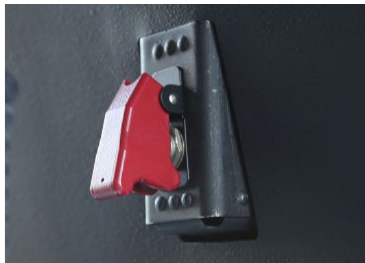
Figure 32. WOG Override Switch
