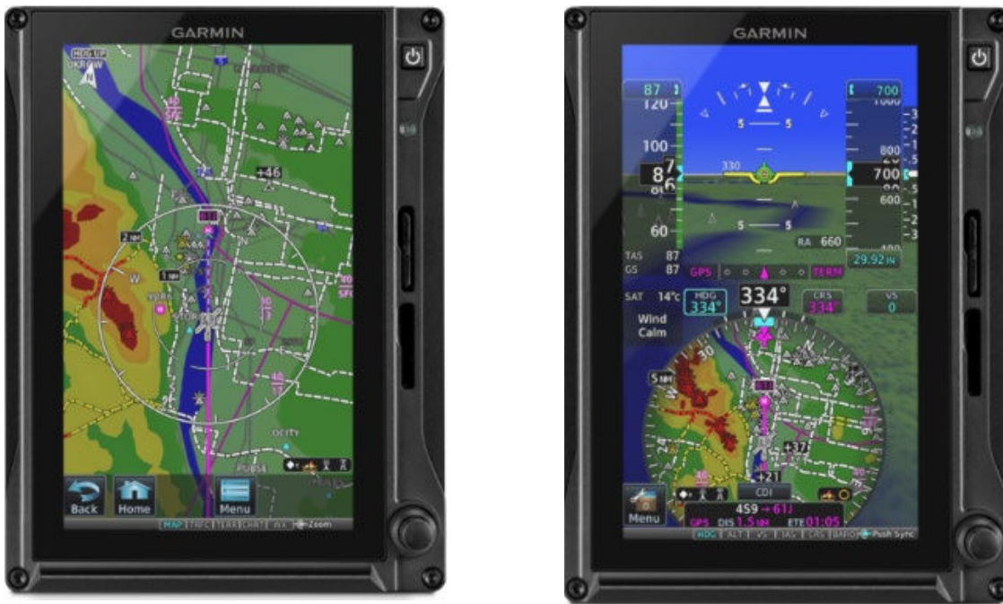
Figure 11 Garmin GDU 700P Touchscreen Displays PFD/MFD
