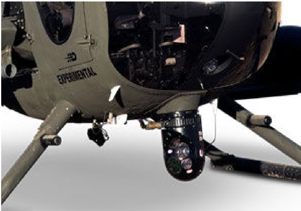
Figure 23. MX-10/10D EO/IR Turret Imaging System
