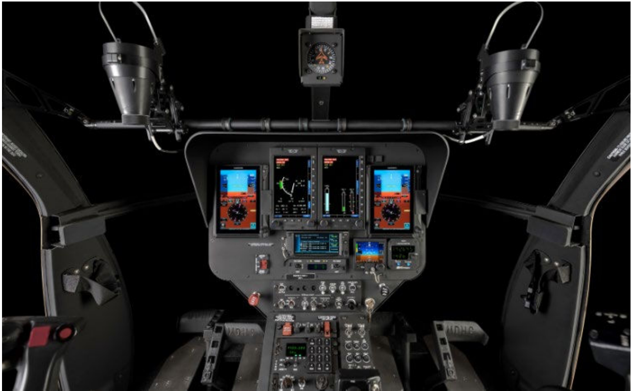
Figure 9. Glass Cockpit with Howell Engine Instruments Display & Garmin G500TXi MFD/PFD
