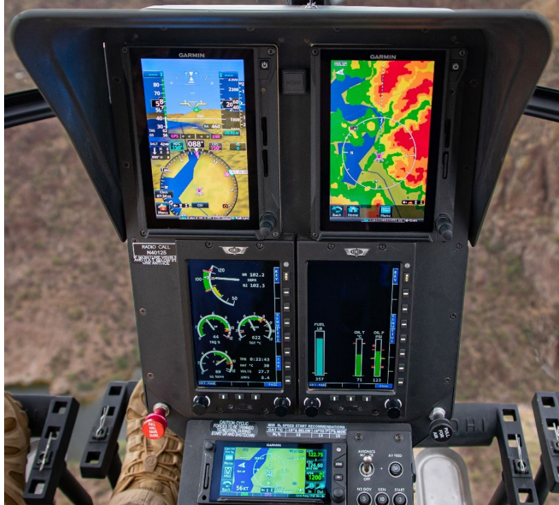
Glass Cockpit with Howell Instruments Engine Instruments Display, Garmin G500H TXi™ MFD/PFD, and GTN™ 650Xi.
