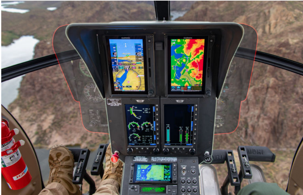
MD's new slimline glass cockpit provides increased visibility on both sides compared to the old analog cockpit design.
